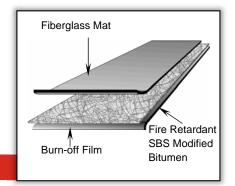
Meets or exceeds performance requirements of ASTM D 6164, Type II, Grade G
