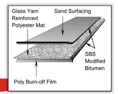
Meets or exceeds performance requirements of ASTM D 6164, Type I, Grade S
