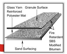
Meets or exceeds performance requirements of ASTM D 6164, Type II, Grade G
