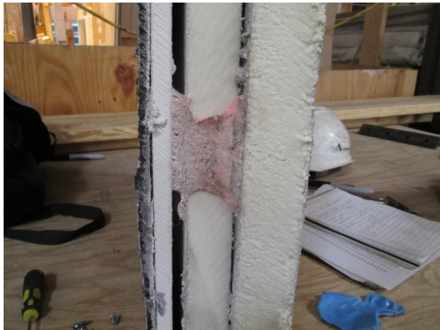
Photo No. 2 Cross-Section of Roof Buildup
