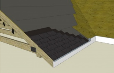
Asphalt Shingled Roofs
