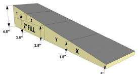
Figure 2. Duro-Guard ISO III CG Taper
