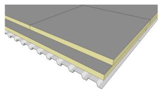
Figure 1. Duro-Guard ISO III CG Flat On Steel Deck
