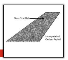
Meets ASTM D 2178, Type IV. Tested in Accordance with D 146.
