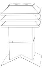
Ridge flashing (SDF)
